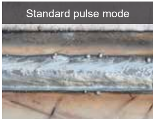
Spatter adhesion and undercut occur.
